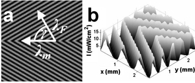
FIG. 1. A mask for spatial periodic forcing of Turing patterns (a) and its calculated intensity map upon projection onto the working medium (b). Vectors represent the primary directions of periodicity with wavelengths  $\lambda_F$  and  $\lambda_m$ .  $\lambda_m$  is a function of the rotation angle  $\gamma$  and  $\lambda_F$ . Intensity surface is chipped due to numerical rounding.
