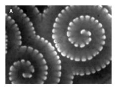
**Spirals and worms.** (A) Segmented spirals emerge from about one million interacting nanodrops of aqueous BZ solution in an oil-water microemulsion (15). Frame size,  $3.72 \times 4.82 \text{ mm}^2$ . (B) In a simulation (16), a BZ gel "worm" autonomously reorients itself to localize in the dark region.
