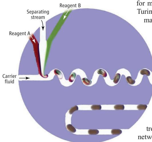
**Microfluidics plus chemistry.** A microfluidic channel carries water droplets of volume 250  $\mu\text{l}$  in a continuous stream of oil. [Adapted from (18)] The droplets act as microreactors in which the reagents are rapidly mixed (upper undulating region) and are then transported with no dispersion (lower smooth region). Such an arrangement can be used to control chemical reaction networks on a millisecond time scale.
