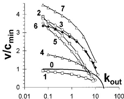
FIG. 5. Dependence of  $\nu$  on  $k_{out}$  for system (2), (5). Parameters  $k_f$  and  $k_b$  are shown in Table II,  $k_a=1$ ,  $K_m=0.01$ ,  $k_t=0.01$ ,  $D_X=0.01$ ,  $D_R=1$ ,  $c_{min}=2(k_a D_X)^{1/2}=0.2$ . Curve 5 represents two nearly identical curves for  $k_f=0.2$  obtained with different values of  $k_b$ . Curve 0 is normalized velocity obtained from Eq. (14), where  $x_1$ ,  $x_2$ , and  $x_3$  are shown in Fig. 4(b).
