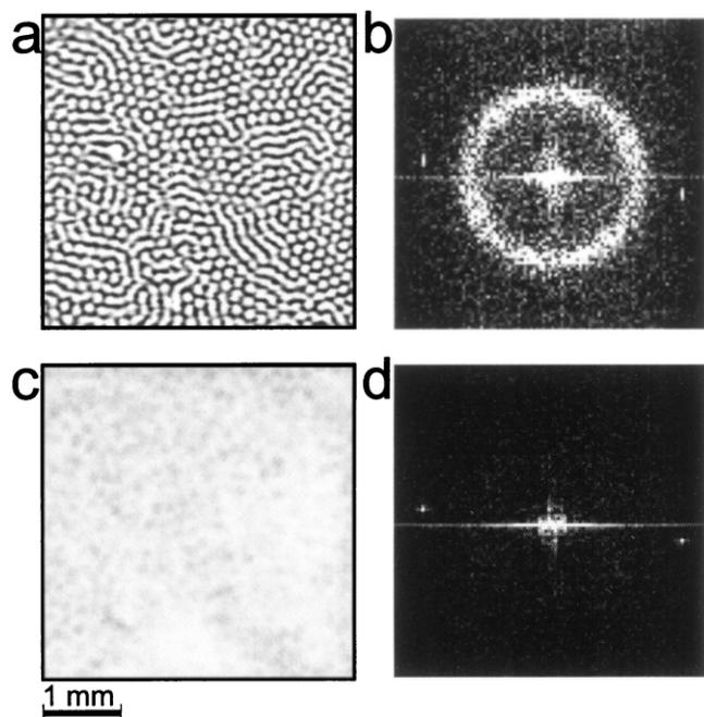
FIG. 1. Suppression of Turing structures with periodic rectangular pulses. Period of illumination is 36 s; light and dark phases have equal duration of 18 s. Light intensity during light phases is 65 mW/cm<sup>2</sup>. (a) Initial pattern at the start of illumination—a mixture of spots and stripes; (b) Fourier spectrum of initial pattern; characteristic wavelength is  $0.16 \pm 0.02$  mm; (c) pattern after 25 min of illumination; (d) Fourier spectrum of pattern shown in (c).
