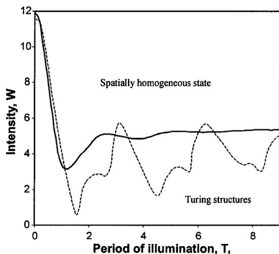
FIG. 4. Resonant dynamics of periodically forced Turing structures in two-dimensional system according to Eq. (1). Boundary between domain of Turing structures and that of spatially homogeneous state is calculated for  $\sigma = 9$  (dashed line) and 15 (solid line), other parameters are  $a = 36$ ,  $b = 2.5$ , and  $d = 1.2$ .
